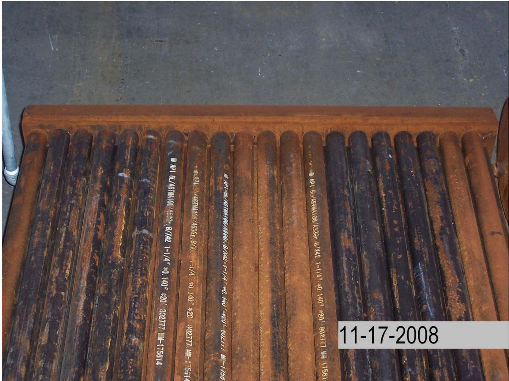
API 6L/ASTM A106/ASME B36.10 1-1/4" #0.140" #20 302777 MM-175614
